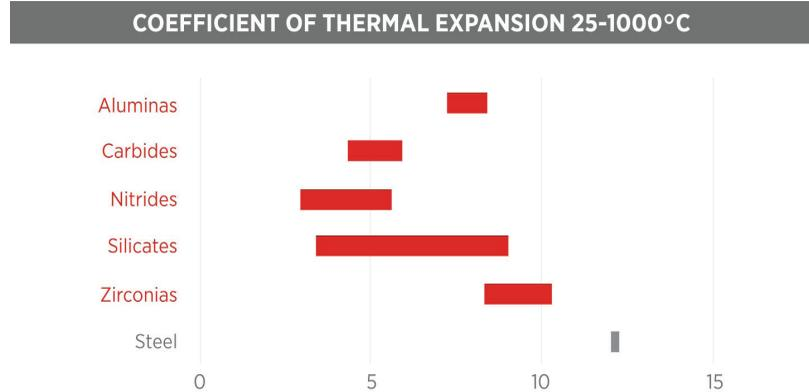
*Technical ceramics have a low coefficient of thermal due to their strong interatomic bonds. The ability to retain material properties in high temperature environments make ceramics a strong choice for sensor components.*
