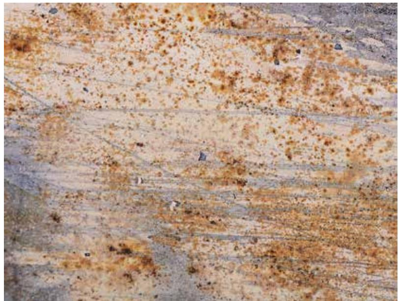
Figure 3 Stainless steel with signs of pitting corrosion
