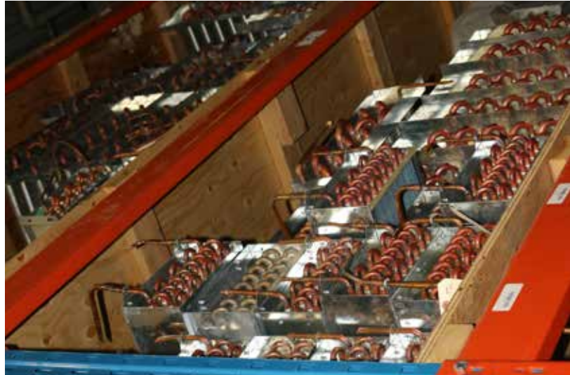
Various MicroGroove heat exchangers in storage. (Courtesy of MTL Technologies)
