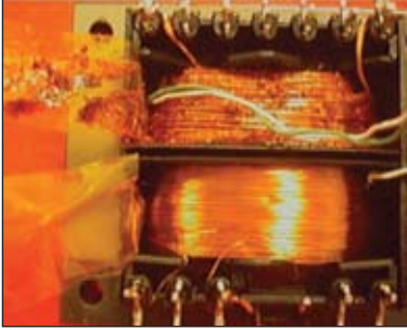
Figure 1. Effect of a secondary short on a 240 VAC transformer utilizing a thermal fuse as the primary protection element.
