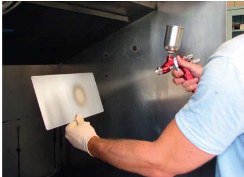
The liquid metal marking material can be applied using conventional spray equipment.
