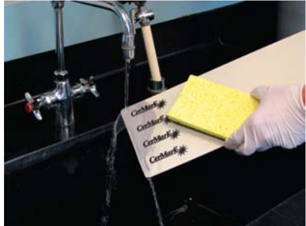
When spray-type marking material is used, the excess can be simply washed away with plain water.
